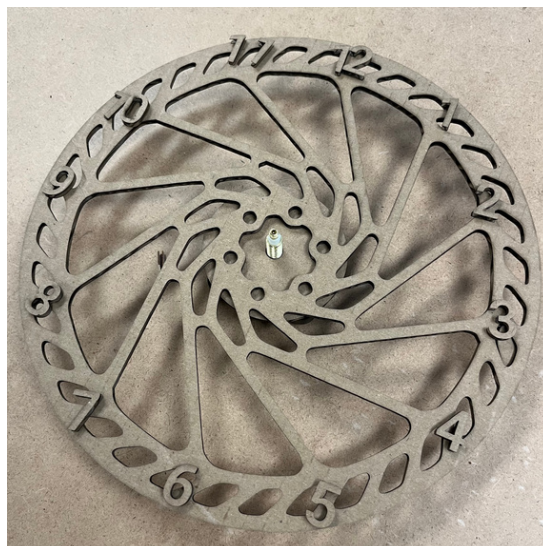
Above is a prototype of the clock made out of cardboard to test the size and shape of the design before acrylic is loaded into the cutter. To the right, you can see a video of the laser cutter cutting silver acrylic for the clock base.
