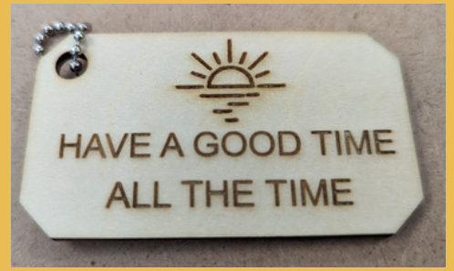
Students learn how the speed and the power settings of the cutter affect the look on materials.
